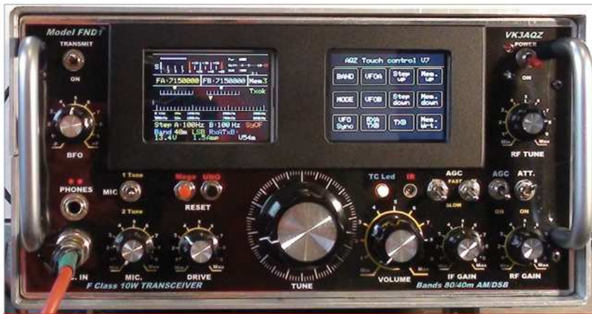
Photo 1. View of the transceiver project's front panel. Microphone input is at lower left.
