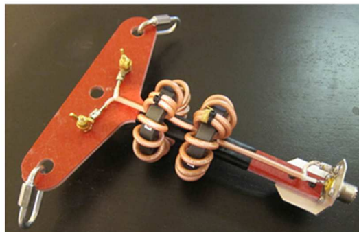
Fig 11 – W6GJB's Dipole Center Insulator With Two RG400 Chokes
