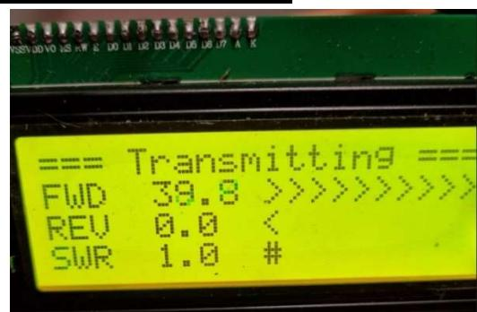
Calibrating is carried out by applying forward power (100W) into a 50 ohm load and adjusting the trim pot on the board so the output is 5.00v. Same steps for adjusting reverse power, only this time the TX and Antenna coax is reversed.
