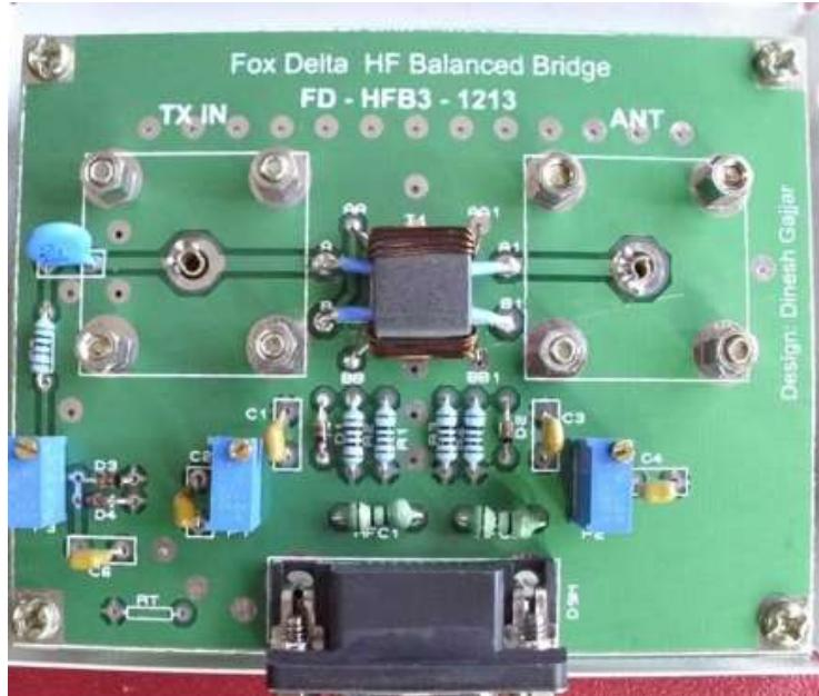
This design utilises a binocular core toroid. Easier than two separate cores.
