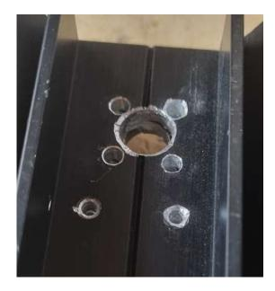
Next, clamp and drill all holes through the second heatsink, sandwiching these together.
