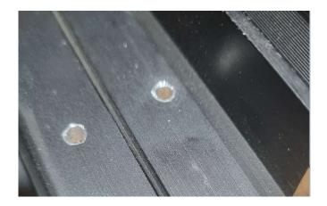
Next to mark and drill the holes for the bulkhead coax connector. I used a BNC here. Make the center pin relatively close to the tab on the resistor. I made this one 15mm apart.
