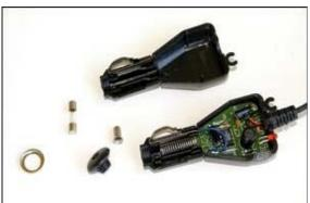
The charger pulls apart really easily – just undo the threaded collar at the pointy end of the plug and then separate the two halves. A fuse will fall out – you can put that in your spare parts drawer and the rest of the housing in the bin.
