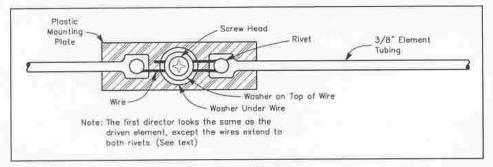
Figure 2-Drawing of the driven-element modification.
