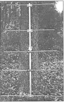
ened. This puts the center of the element at the same electrical potential as the boom. Using the 1½-inch pigtail, bend it and place it between the two washers so there is a piece of wire on each side of the bolt. This prevents the washers from tilting and makes for a cleaner fit. Trim off any excess wire. (All of the foregoing is more difficult to describe than it is to perform! It doesn't take long to do once you understand what is going on.)
