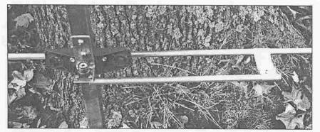
Figure 6—The gamma match and driven element.
