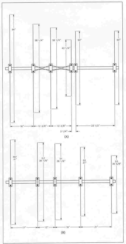
Figure 1—At A, the original configuration of the RadioShack FM receiving antenna. The element lengths and spacings at B are chosen for operation on 144 MHz. For operation on higher frequencies, shorten the elements even more; see text.
