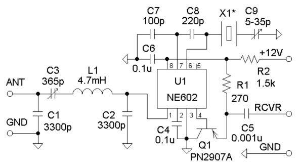
\*X1: Any desired frequency from about 2 to 20 MHz
