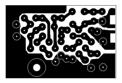
**Printed Circuit Board Solder Side.**
