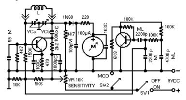
All resistors = 1/8 watt Capacitors C = Ceramic M = Dipped Mica ML = Mylar
