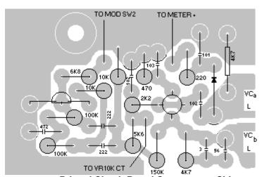
**Printed Circuit Board Components Side.**
