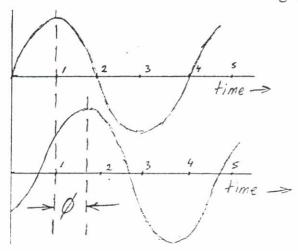
Two similar signals (frequency and amplitude the same but differing in phase.
