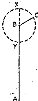
◆ Fig. 1—The mechanism by which the undesired side frequency makes a "ripple" on the desired side frequency of an s.s.b. signal. Other possible spurious components are neglected in this drawing, but can be included if their relative amplitudes, phases, and frequency separation from the desired side frequency are known. ◆
