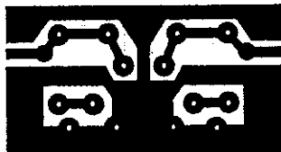
Circuit-board etching pattern for the 144-MHz stop-band filter. Black represents copper. The pattern is shown at actual size from the foil side of the circuit board.
