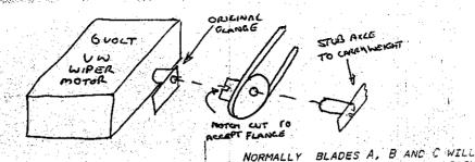
THE NEXT PROBLEM IS HOW TO LIMIT THE ROTATION OF THE DRIVE SHAFT, SO THAT YOU DON'T KEEP WINDING THE SHAFT ROUND AND ROUND, RESULTING IN DAMAGE TO THE COAXIAL CABLE. SHOWN BELOW IS ONE WAY TO DO IT:
