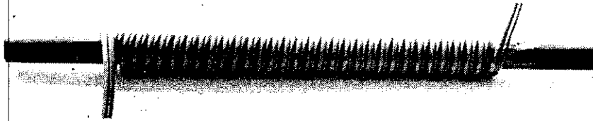
Interference pickup on speaker leads may be cut by winding part of the lead, nearest the amplifier terminals, on a ferrite rod — available at many parts suppliers.
