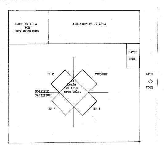
The centre of the 4 operating tables consists of a square of wooder partitions to about 8' high. These will be a map, clock and speaker mounted on each. All cables to and from the operating positions will go into this middle section from where they will go either overhead or under the floor to the patch desk. All patching will be done at the patch desk so that there is no need for the operators to get to the cables behind the equipment and the boys can not get to the connections either.
