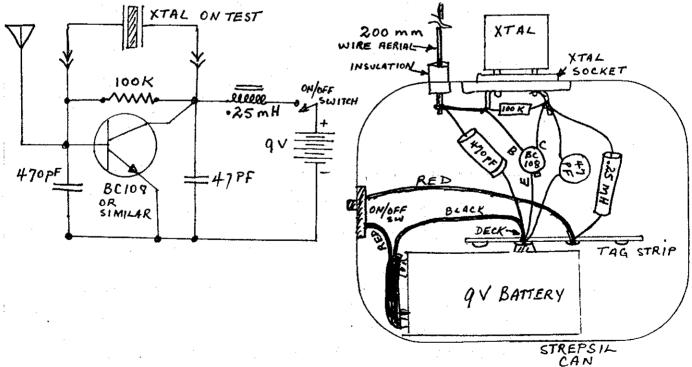
This device is especially useful in tuning up a VHF transceiver. Proceed as follows:
