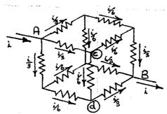
resistors are 1 ohm apply Kirchoff's Current Law to show that a current of i/3 amps flows through each branch connected to A. Continue to apply KCL for each node to obtain all currents as above.
