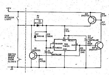
This time delay circuit is easily adaptable to turning off an alarm system and resetting it after a preset period. The values shown will keep the load activated for about 10 seconds, but can be adjusted for values up to many hours. Reprinted from LIMARC Log.
