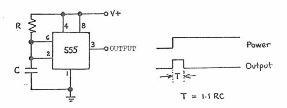
If a 555 is connected as shown, the device will self-trigger when the power is turned on, and will complete a single timing cycle. At turn-on, C is discharged, which momentarily holds pin 2 low, beginning a timing cycle. Capacitor C then charges up to V+ through R, and when the voltage crosses 2/3V+, the pin 6 threshold is reached, which completes the cycle.
