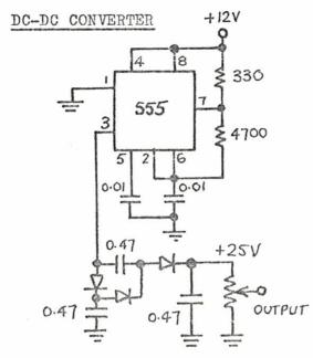
This circuit allows maximum use of the tuning varactor.
