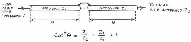
For a 50/75 ohm transformer this works out to an electrical length of 29.3° for each section of cable; the physical length must take into account the velocity factor of the cable (typically for coaxial cable around 0.66).
