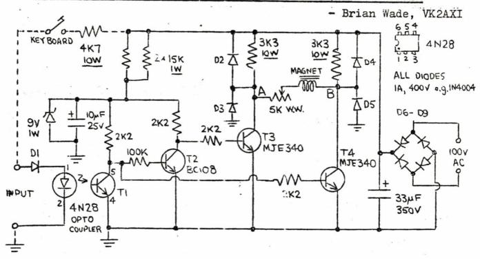
This circuit provides double current drive for a Creed receiver magnet, and requires only a single 100-110 volt AC supply to power it. Signal input is by opto-isolater, so a current of 10-20 mA from any source into the LED will operate the magnet driver.
