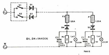
lamps, which therefore burn at normal intensity. The value of these capacitors is determined by the power rating of the lamps used. The appropriate value can be calculated by using the following equation:
