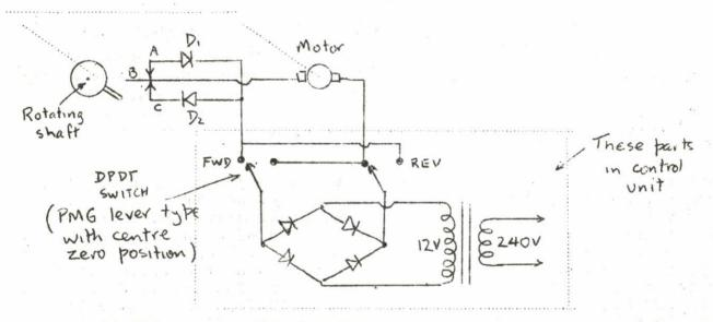
With the operating switch in the FwD position, current flows from power supply through motor, along blade B, into blade A and back through diode D<sub>1</sub>. Motor rotates shaft clockwise until lug depresses blade B, bending it away from blade A. Motor stops because path via blade C is blocked by diode D<sub>2</sub>. But motor will run in reverse from this position, because diode D<sub>2</sub> will now conduct when polarity of supply is reversed.
