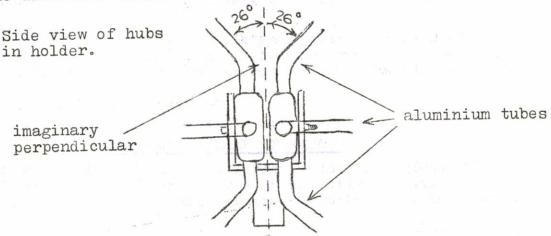
Eight 15 feet fibreglass fishing rod blanks were then used. They slide perfectly onto the 1 inch aluminium tubes. Ensure that the tubes are all exactly the same distance and angle between each other. Then secure them to the hubs. The fishing rods are then slid onto the aluminium tubes and then secured by using fibreglass tape, resin and hardened. This completes the basic construction.
