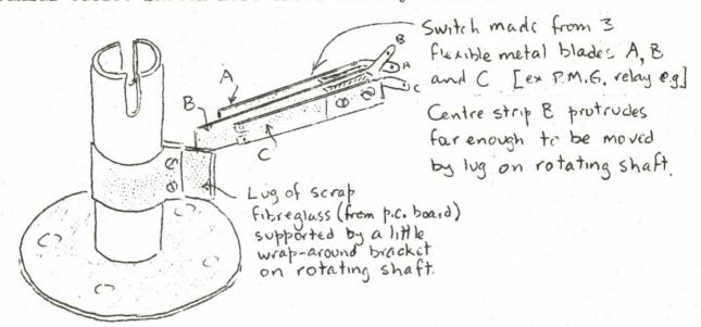
Normally blades A, B and C will be in metallic contact with each other. But when the shaft rotates far enough, the protruding lug of fibre-glass will bend lug B aside until it no longer contacts lug C (if rotating clockwise) or lug A (if rotating anticlockwise). Add two heavy duty diodes (I used automotive press-fit types ex junk box) and a reversing switch in the control unit, and you now have automatic travel limiting:
