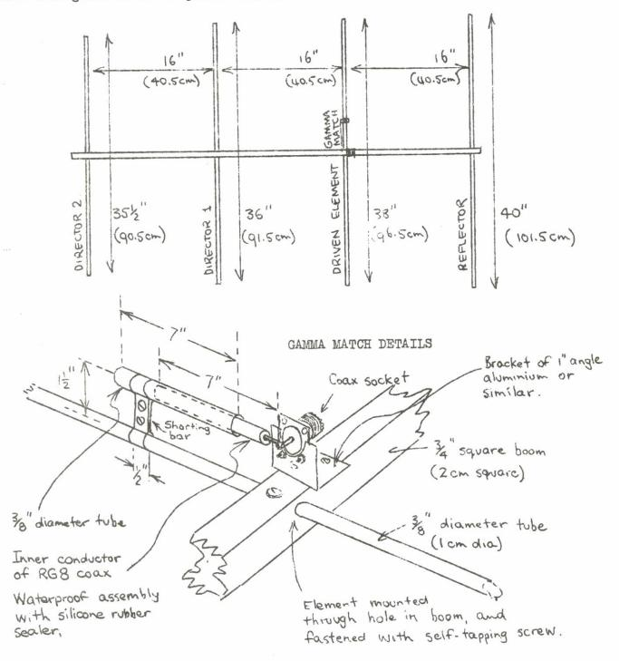
The four elements and the gamma bar can be cut from two lengths of 2-metre long tubing. The square boom makes construction easier than would be the case with a round boom. Aluminium or wood can be used for the boom.
