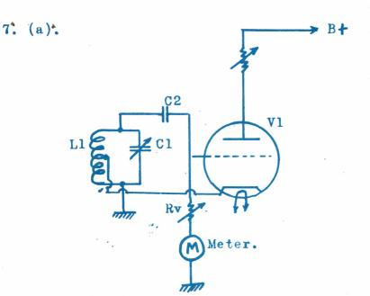
Valve V1 operates as an electron coupled oscillator. As such, it draws a certain amount of grid current, indicated on meter M. When Ll is coupled to another tuned circuit of the same frequency, that circuit will absorb some of the energy from the oscillation. Oscillation will be reduced, hence grid current will be reduced & the meter "dips". If Cl is calibrated, the frequency of the unknown circuit can then be determined from the scale.
