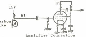
Variations in resistance cause the current through the mike & RI to vary Hence the voltage drop across M varies This audio voltage can be applied to the grid and amplified normally. Alternatively, the grid can be grounded and the mike connected between cathode and ground.
