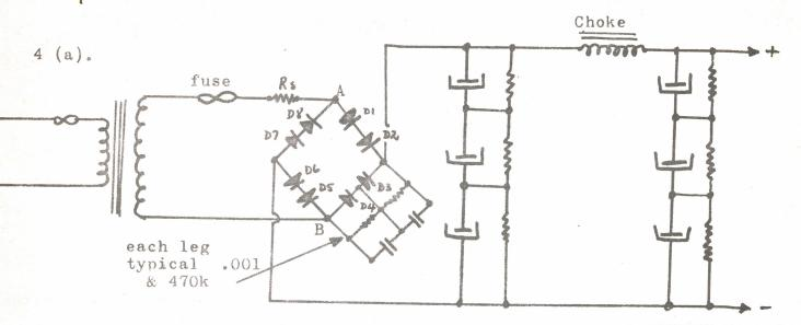
During that half cycle when point A is positive in respect to point B, current will flow through diodes  $D_1$   $D_2$  &  $D_5$   $D_6$ .
