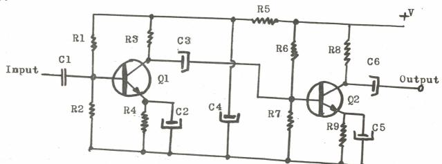
The input is AC coupled to the base of transistor Ql via Cl. Cl should have a large enough value to present a low reactance at the lowest frequency
