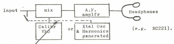
The incoming signal is mixed with the known signal from the calibr. VFO. When zero beat occurs, the unknown frequency equals the known frequency ii. from the VFO. (calibrated dial readout).
