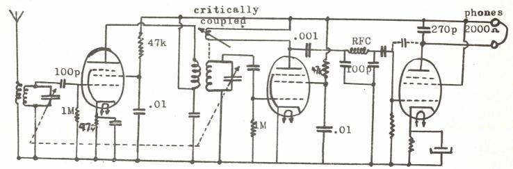
(i) RF Amplifier amplified at signal frequency. (ii). Regen. Detector produces audio at the plate due to non linear action. (iii). Pie filter (RFC + 2x100p) blocks RF. passes audio to amplifier.
