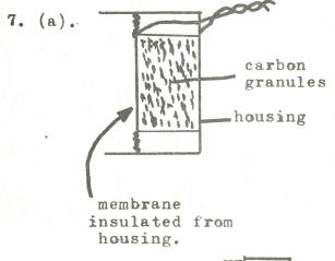
Speech moves the membrane, compressing & de-compressing the carbon granules. The resistance will vary with sound pressure and frequency.
