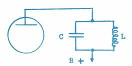
When the L C tuned circuit is not in resonance, the HT flowing to the anode, only sees the DC resistance of coil L, which could be a few ohms. When L C is brought into resonance, the resistance of the network could increase to a couple of thousand ohms, hence a drop (dip) in anode current.
