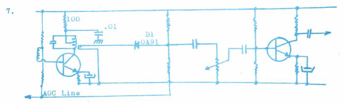
When 455 KHz IF signal is present, rectified DC will appear after diode Dl. This negative voltage to the bottom of the voltage dividers for transistor bias can reduce the transistor gain according to the strength of RF. (IF Sig).
