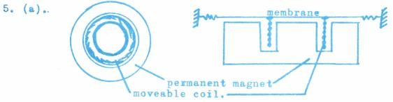
Sound waves striking the diaphram cause movement of the coil thru the permanent magnetic field, thereby generating a voltage.
