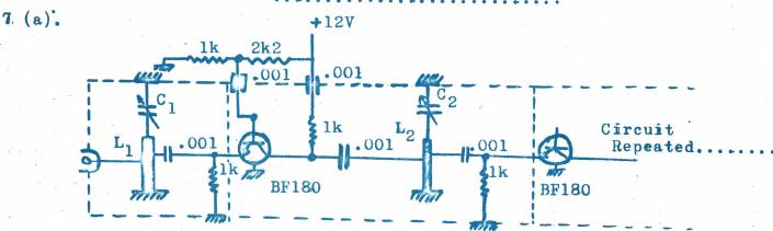
Stripline 432Mhz RF Amp. L<sub>1</sub> resonates within C<sub>1</sub> in its cavity on 432 MHz. ditto for L<sub>2</sub> & C<sub>2</sub>. Input circuit is tapped to give correct input impedance as is .001 pF tap to feed transistor. This particular circuit is referred to as grounded base.
