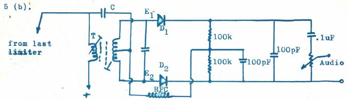
FM is converted to AM in transformer T. V = 90° out of phase with the primary current. Primary voltage is added...... at centre tap.... to secondary via C & combines so that the voltages on each side of the centre tap.lead and lag an equal amount. After rectification they equal voltages but opposite polarity, hence cancel out. When frequency changes, instantaneously E decreases while E increases & vice versa, producing a change in voltage (amplitude) & audio.
