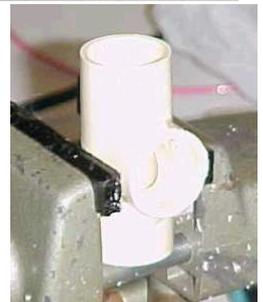
Now cement this "T" (un-trimmed side) to the other end of that 533mm length of CPVC tubing as outlined at the end of "Part 2", On the other side of the "T" (un-trimmed side), cement a 300mm length of 19mm CPVC.
