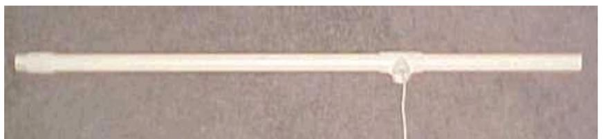
**NOTE: PAST THIS POINT, YOU MAY WISH TO REFRAIN FROM CEMENTING THE CPVC WHERE INSTRUCTED IN CASE YOU NEED TO MAKE ANY CORRECTIONS TO YOUR WORK. AFTER THE ANTENNA IS COMPLETED AND TUNED YOU CAN CEMENT ALL REMAINING JOINTS (Just don't forget any)**
