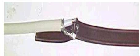
Measuring exactly **38mm** from this connection, remove 1.5mm of insulation from each wire in the twinlead by melting to expose the wires. At this point, solder one end of the coax with the centre conductor going to one wire and the shield going to the other as
