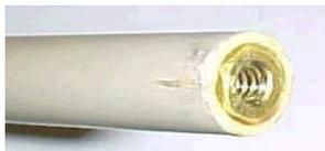
Snake the 1120mm of wire through a 965mm length of the 12.5mm CPVC tubing. Roughen up the inner portion of the tubing near where the nut will sit. Epoxy the nut so it's pressed into the tubing but **flush** with the end of the tubing as shown. Do not get any epoxy on the nut threads.
