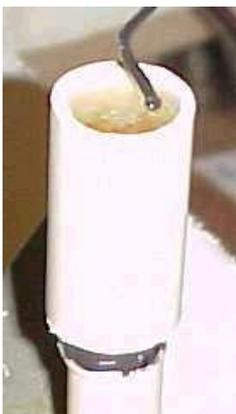
Insert a shim of cardstock around to fill the small gap between the smaller CPVC and the sleeve as shown in BLACK on the photo to the left. This keeps the entire assembly straight after the epoxy has set so you'll be able to easily unscrew the top (thinner section) from the lower section.
