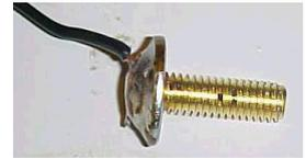
3. So, now you have a screw with a soldered washer and a wire soldered to the top. Now cut a cardboard circle slightly wider than the inner diameter of the 19mm CPVC tubing and cut a centre hole so the cardboard washer fits snugly on the screw .
