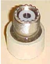
Cut a 1/2 piece of the 19mm CPVC tubing from your remaining stock and sand both ends flat. Sand, to roughen, the inner section of this piece. Laying it flat on a piece of card stock, place the barrel connector exactly in the middle of the tubing and pour epoxy into the gap as shown. Be careful not to get epoxy on the exposed threads.
