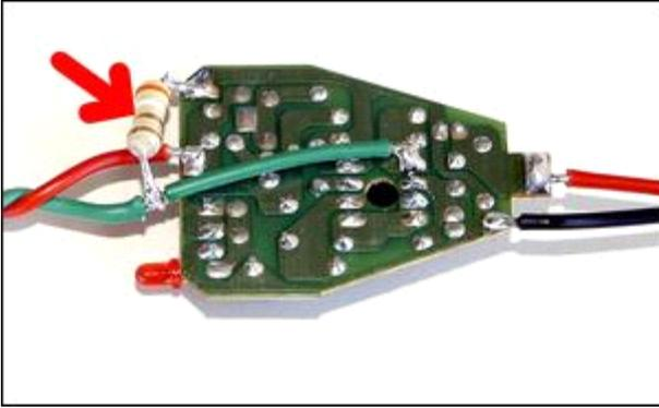
Making sure that you're working on the output side of the module (that's the non-pointy end), solder the new 3.9 ohm 1 watt resistor between the green wire (the new one that connects to Pin 5) and the negative output (black). In this view the negative wire got so short it's lost its black insulation.
