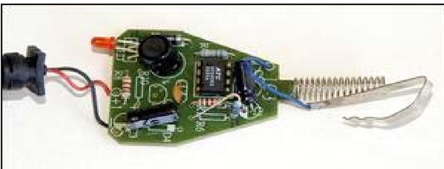
Here's what the bare guts look like. Note the red and black wires on the left – they're the positive and negative (respectively) power outputs. The inputs are on the right – the spring that connected to the tip of the plug is positive and the other wire, negative.
