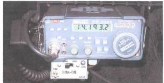
Figure 6—The Tenna Tune installed with the author's SGC-2020.
